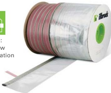
TP601 is a weather-retardant, impregnated, open cell, polyurethane soft foam, enclosed before use in a polypropylene film with a bonding adhesive on one side for fixing.
