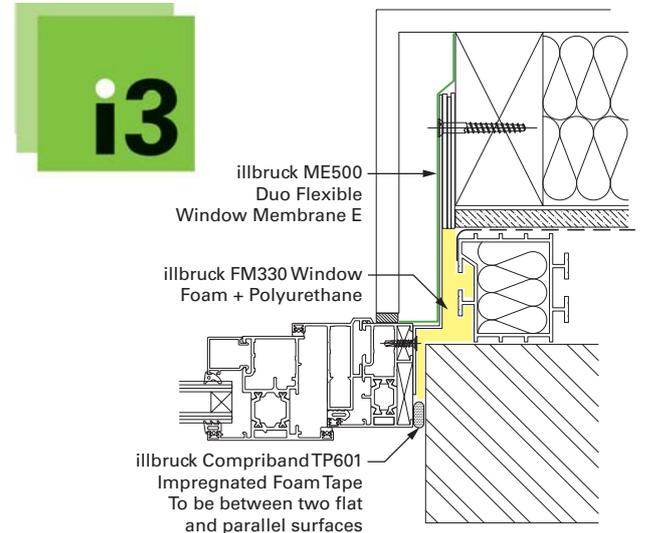
Timber Frame detail at jamb showing full i3 solution to provide an effective weatherseal, thermal insulation and air tightness after settlement.
