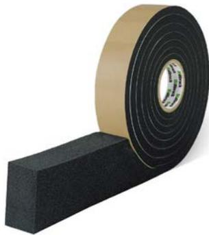
A soft and flexible open cell polyurethane foam, impregnated with an acrylic based, UV stabilised resin. The resin is water repellent and contains a fire retardant. TP450 has a self-adhesive side to aid initial location and is easy to apply in any weather. Additionally, TP450 has both thermal and acoustic insulation properties. TP450 is designed for use in a wide variety of movement joints up to 50 mm wide and can accommodate up to 37 mm of movement.
