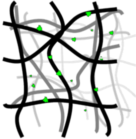
Diagram of electrostatic filter
